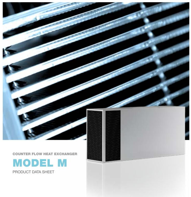
Model M is a high-efficiency counterflow plate heat exchanger, specially designed for the demanding requirements of the telecommunications and electrical enclosure industry. Even in a dry situation, it can come close to 90% (sensible) efficiency.
